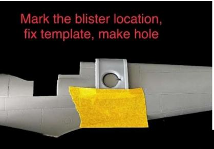
Hatches & Blisters: Use the corresponding template to mark the position, align the inner ribs of the fuselage with the slots on the template. Once satisfied, attach temporarily the template with tape. Drill multiple holes and finish with scalpel to remove the inner portion. Finish with flat and round files to conform to the template opening. Check the fit of the hatch/blister with your opening regularly, but again, don't force it into, it would break.
